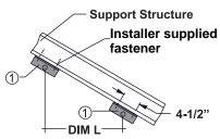
**DIM L = Distance between mounting** holes. (Refer to owner's manual)
