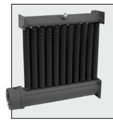
The *ExCaliber*<sup>™</sup> vacuum sealed liquid-to-air heat exchanger core is constructed using rugged, copper-free, roll-formed aluminum fins and protected by a pressure relief device, automatic reset high limit, and a back-up manual reset high limit.
